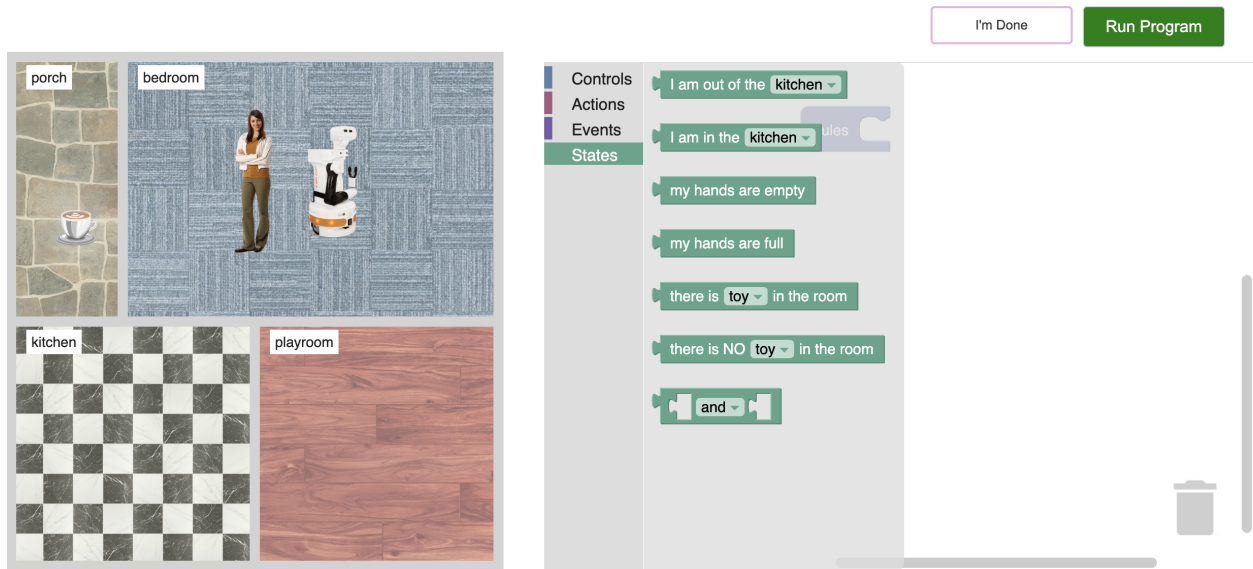
Figure 8: The graphical interface in Blockly for Trigger-Action Programming (TAP) with the State blocks displayed in the coffee delivery task (Task 4).
